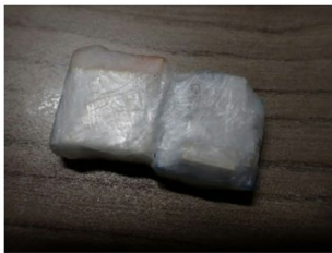
Fig. 1 Images of A the accelerometer unit, B the accelerometer unit packaged within layers containing zip-lock bags and Parafilm, and C individual P. megacephalum affixed with the accelerometer unit via epoxy putty glue
