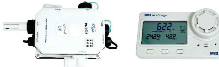
Figure 1: a) DL-1038 (left); b) HOBO MX1102A CO 2 (right) data logger.
